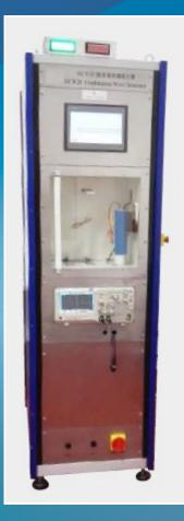
Surge generators can be used to generate impulse of exponential shapes to perform high energy surge tests. The system can output combination wave (open circuit voltage  $1.2/50\mu s$  & short circuit current  $8/20\mu s$ , open circuit voltage $10/700\mu s$  & short circuit current  $5/300\mu s$ ). With additional impulse modules, it can output  $10/350\mu s$  and  $8/20\mu s$ .
