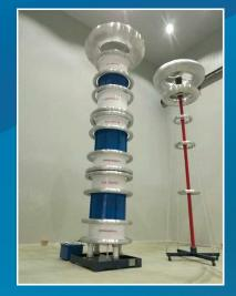
AC resonant test systems with variable inductance and module type are used for factory testing of medium and high voltage cables, power transformers, bushings, high voltage capacitors, generators, arresters and high voltage accessories. They include stackable modules that can be used to test a wide range of products. The systems can be expandable to cover future test requirements that may require higher voltage and power levels.
